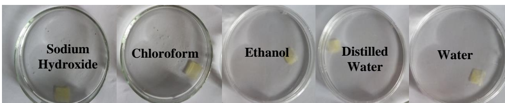
Figure 3: Solubility test of membrane in 1 M NaOH, \text{CHCl}_3 , EtOH, distilled water and water
